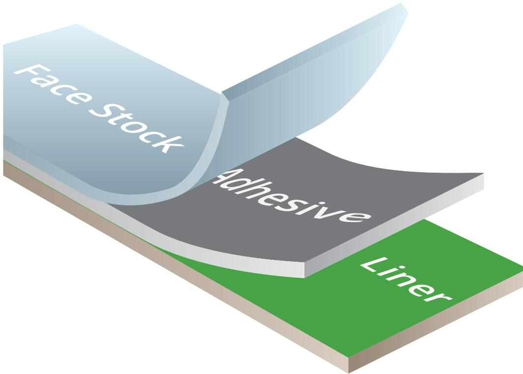
**Face Stock:** 2.4 mil topcoated matte white polyimide film offering excellent chemical resistance combined with superior high heat resistance. The material will not curl and is designed to survive high temperatures of lead-free solder processes.
