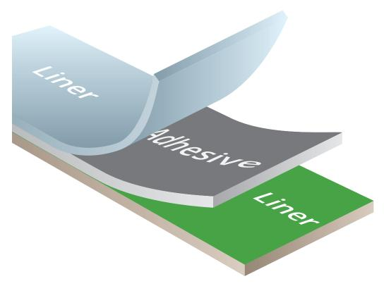
**Release Liner:** Available with a 4.2 mil 58# polycoated kraft double liner for adhesive cut-outs or adhesive only parts.
