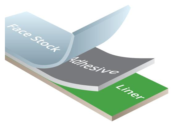
**Face Stock:** 2 mil topcoated gloss white polyester offers excellent abrasion and harsh chemical resistance. The material performs best on the topside of a circuit board where heat exposure is limited. The material will not shrink and is designed to be UV flexographic and thermal transfer printed
