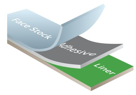
**Film:** 3.2 mil direct thermal matte white polypropylene. Great material for product identification where the product is not exposed to high heats. This material can be used for blank or pre-printed labels.
