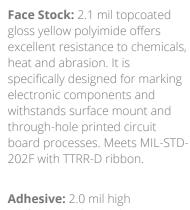
**Adhesive:** 2.0 mil high performance heavy duty permanent acrylic adhesive offering excellent chemical, heat and abrasion resistance.
