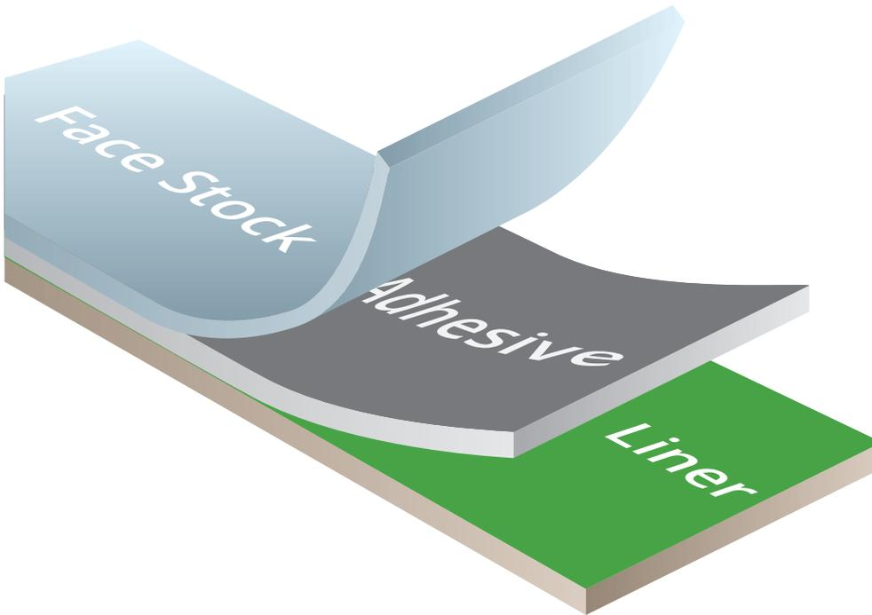
**Face Stock:** 2.4 mil topcoated gloss white polyimide film offering excellent chemical resistance combined with superior high heat resistance. The material will not curl and is designed to survive high temperatures of lead-free solder processes.
